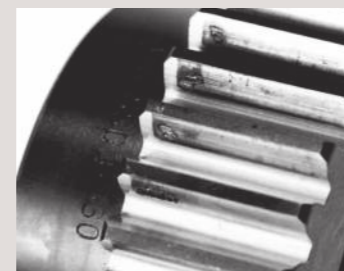
Poor tooth contact and pitting
