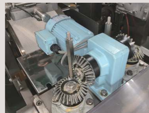
SMB miter used for filleting fish
