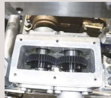
SS spur gears used for filleting fish
