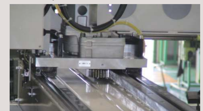
KRG Ground Rack used as a workpiece conveying device
