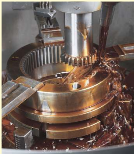
Gear cutting by CNC Gear Shaper
