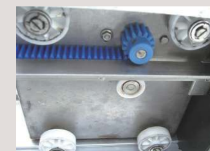
PR plastic rack used for feeding Long Strip Cutter
