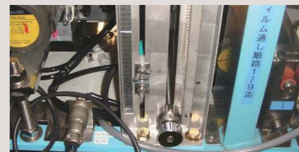
SUR stainless steel rack used for film winding tension part
