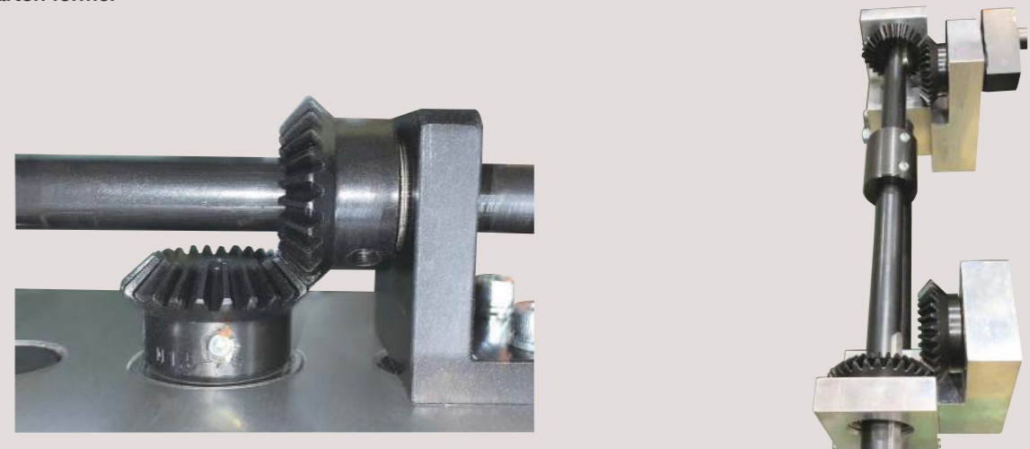
SM and SMB miters used to drive X/Y axes and transmit mechanical power
