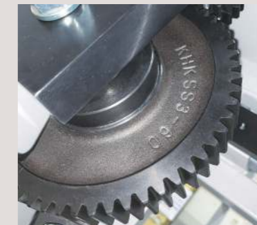
SS spur gears used in automatic carton formers
