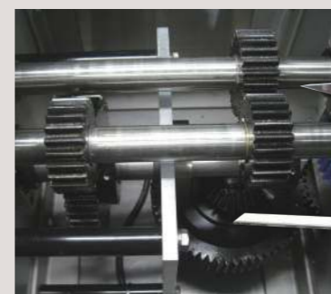
SSA/SS spur gears used in stirrers
