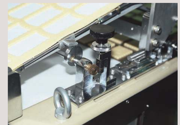
SW worm and BG worm wheel used for adjusting height
