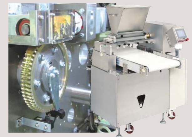
KWGDL Duplex Worm Wheels and AGDL Worm Wheels used for indexing and driving, for accurate filling of a fixed amount of ingredients
