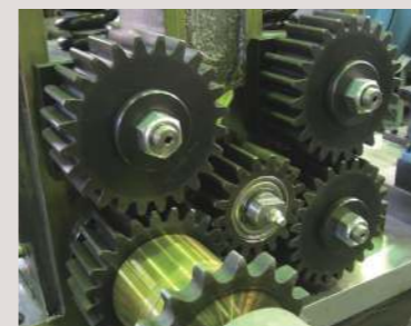
SS spur gears used for wire feeder
